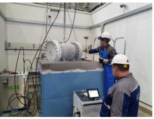
▲ Arctic LNG-2 GBS, axial check valve according to API6D RA 6″-16″ 300RF CF8 36 pcs.;
