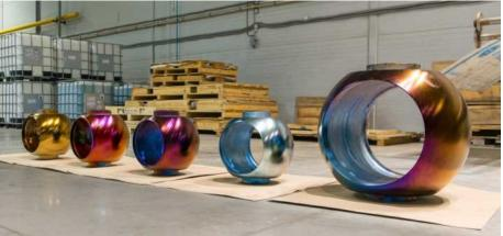
KONAR became the first Russian company, which started to use nickel-plating technology as a protective coating for products.
