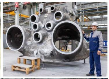
Castings of large pump casing, pipeline valves up to 30 t
