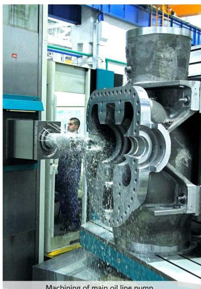
Machining of main oil line pump cover MOL 10000
